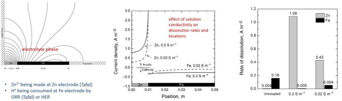
• Shortest path for ions to travel is at junction of the two metals.
